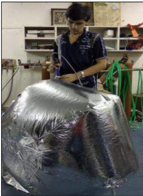
Figure 11. Helium Leakage Test
