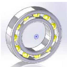
Figure 7: CAD Model of Selected Bearing
