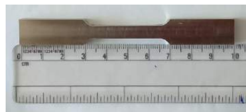
Figure 3: DMLS printed Tensile Specimen
