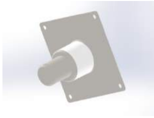
Figure 17: CAD Model for Base Shaft
