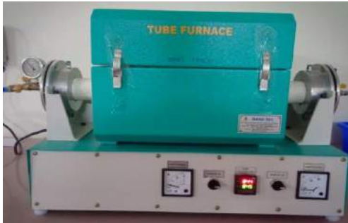
Figure 4: Tube furnace used for Heat treatment
