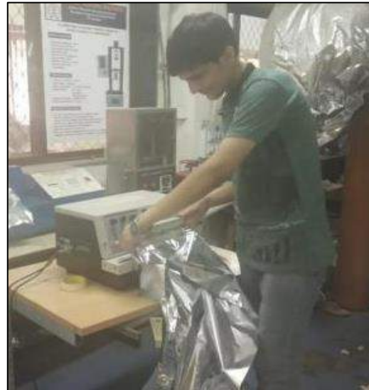
Figure 4. Heat Sealing the Petals
