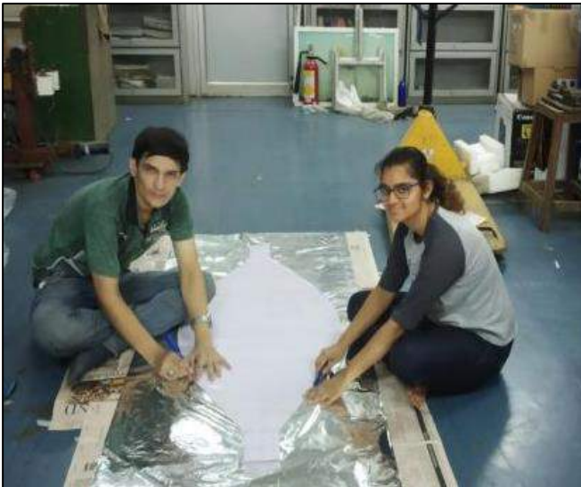
Figure 3. Cutting of Petals on MPET Material
