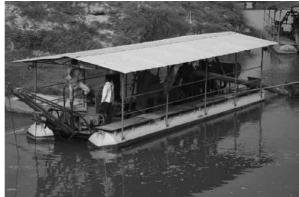
Figure 3 : Suction dredger for alluvial rivers
