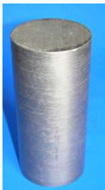
Fig. 6: Typical electron beam double melted niobium ingot of 50 mm dia × 130 mm size.
