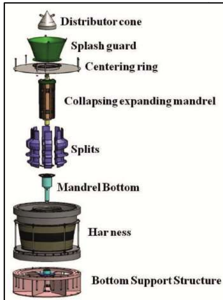
Figure 2.4: Exploded View of CEM
