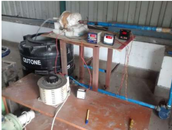
Figure 3: An experimental setup for thermal autofrettage of cylinders
