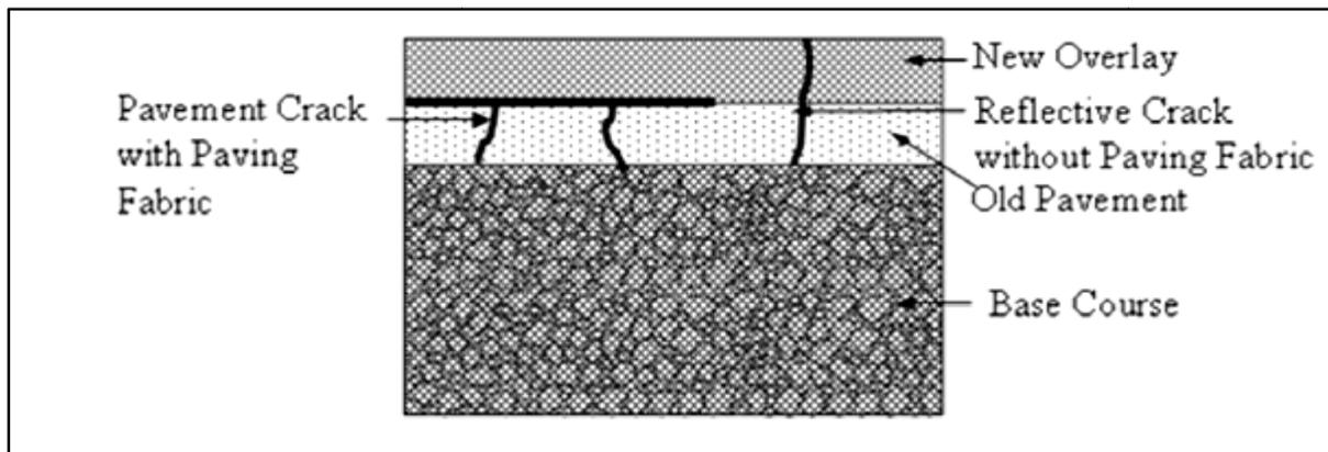
Figure 1 Application of Strain Absorbing Membrane Interlayer (SAMI)
