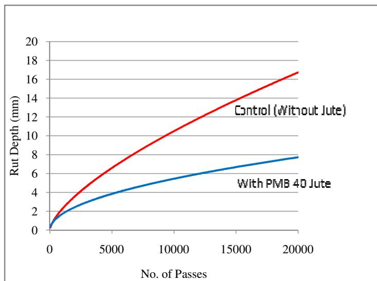
Graph 2: Number of Passes Vs Rut Depth (in Wheel Tracking Test)
