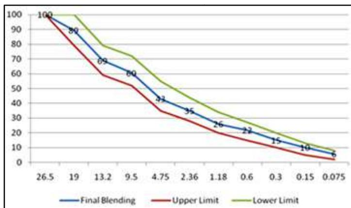
Graph1: Proportioning of Aggregates for BC Mix Design
