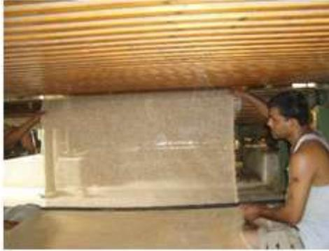
Photo 4: Combination of the combined layers of fabric with woven fabric layer
