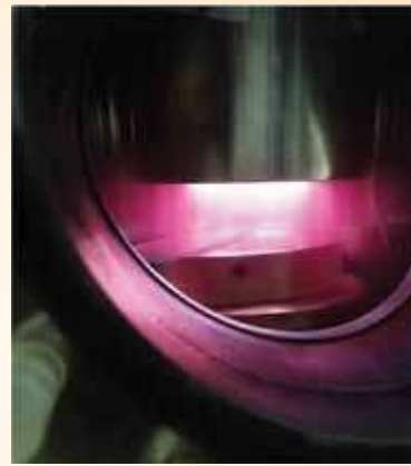
Fig 2: Sputter Deposition of Transition Metal over glass substrate (Courtesy: https://sites.google.com/view/iem-amrl/facilities )
