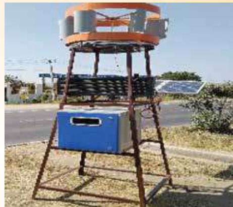
Hybrid PV and plastic bladed vertical axis wind turbine
