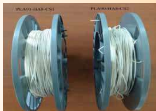
Fabricated feedstock filament of composition (PLA91-HA8-CS1 & PLA90-HA8-CS2)
