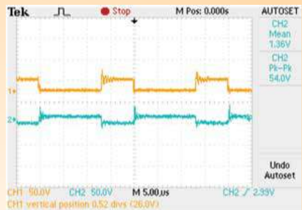
Voltage and Current Waveform across Main Switch with Zero Voltage Transition
