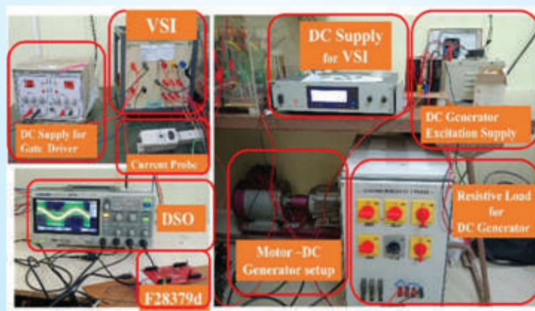
Open-Loop Testing of the Induction Motor Drive for Water Pumping Applications
