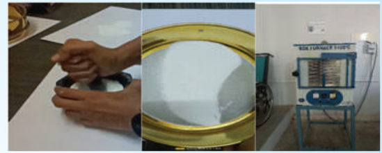
Synthesis of Strontium-doped Hardystonite using sol-gel method
