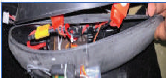
Figure 9: Installed propulsion and wiring system inside the fuselage
