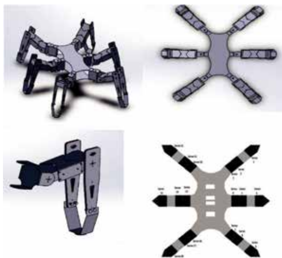
Figure 1. (a) Hexapod CAD model using Solid Works software. (b) Top view of Hexapod CAD model. (c) 3 DOF Arms view of hexapod and, (d) Servo motor position setup using Code: Blocks software in OpenGL mode design
