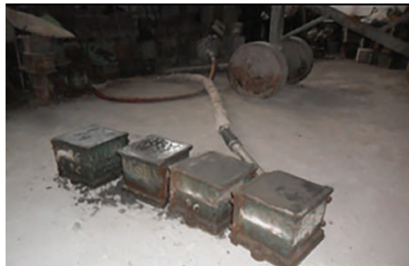
Fig 1 Casing of Concrete cube by compaction with needle vibrator
