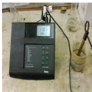
Fig 4 pH value determination of RHA blended OPC
