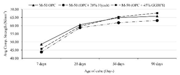
Figure 2 Development of strength over different ages of concrete for M-50 grade
