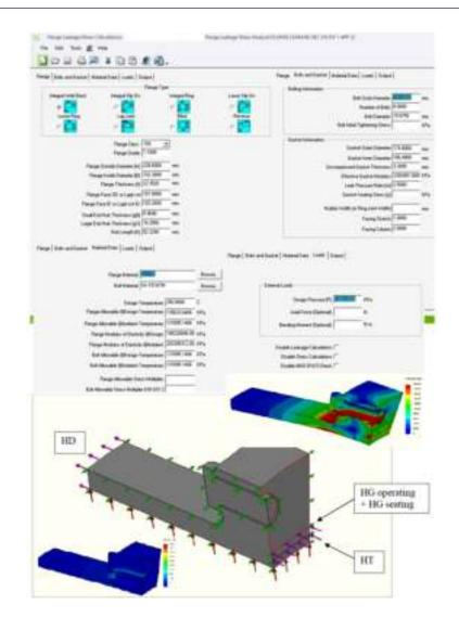
Fig. 4 Flange Evaluation using ASME SEC VIII DIV 1 APP 2 Method
