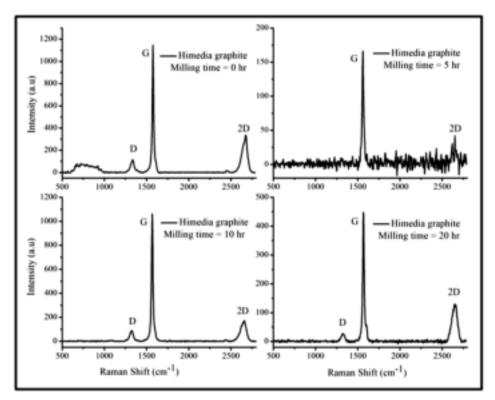
Figure 4 Raman spectrum of commercial graphite
