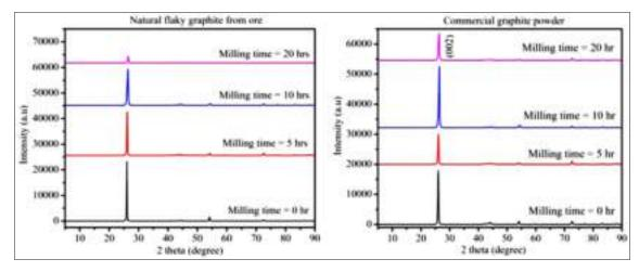
Figure 1 XRD of ore and commercial graphite
