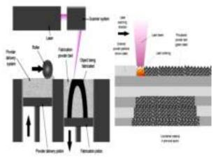
Figure 4 Selective laser sintering
