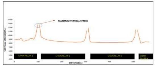
Figure 12 Vertical stress distribution on chain pillars
