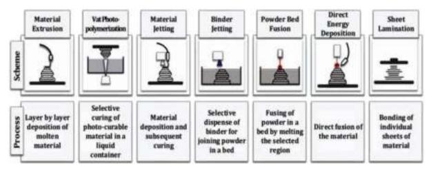
Figure 2 Types of 3D printing technologies and processes
