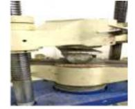
Figure 3 Test set up of split tensile test
