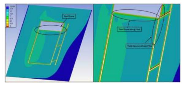
Figure 18 Yield zone in the chain pillars and longwall panel
