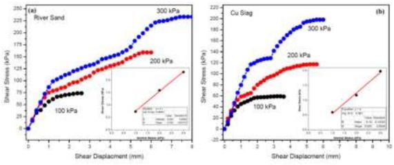
Figure 4 Direct shear test analysis of (a) river sand and (b) Cu-slag
