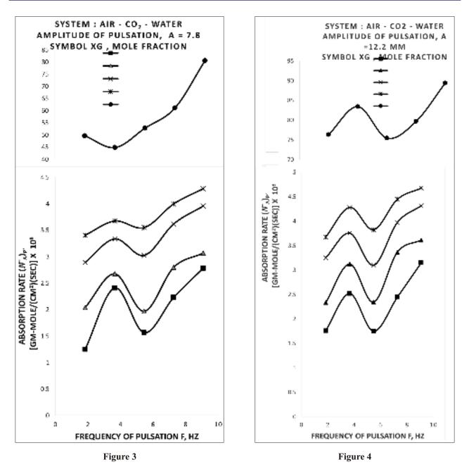
pulsation gives an increased absorption rate when the time period of liquid phase and gas phase oscillation matches. This is completely in agreement with the observation of several investigators [1-3, 7,12]. For  $CO_2$  system the resonance phenomenon shows a 90° degree shift in peek values attainment at amplitudes higher than 21.3 MM. For a gas film controlled process like ammonia water system this is observed at still earlier amplitudes of 15 MM.
