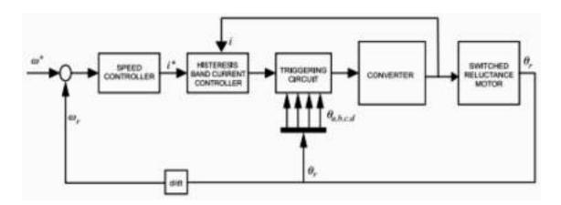
Figure 3 Speed control block diagram of SRM
