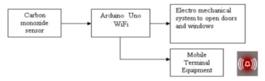
Figure1 Block Diagram of intelligent door and window opening system
