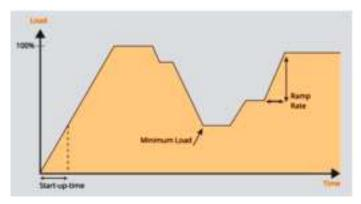
Figure 5 Dimensions of flexible power plant operation
