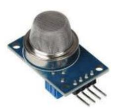
Figure 3 MQ-2 gas sensor
