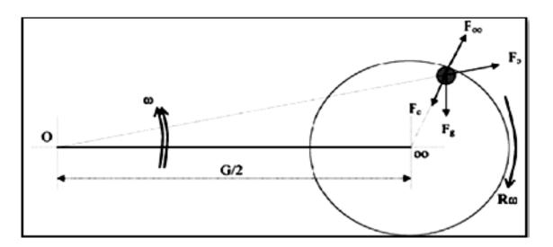
fixed, it turns out, that the planetary mill could be simply characterized by the ratio of the diameter of rotation of the mill axis G to the diameter of the mill D. Let R be the ratio of speed of rotation of the mill axis to the speed of rotation of the mill about its center. Then, if the shaft rotates at an angular velocity of  $\omega$ , the mill rotates at R $\omega$  on the shaft. A negative value of R indicates that the mill and the shaft rotate in opposite direction.
