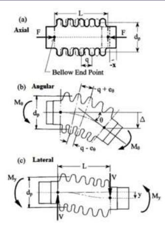
Figure 3 Bellows under deformation [1]
