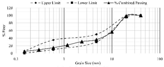
Figure 1 Grain size distribution curve for all-in-aggregates
