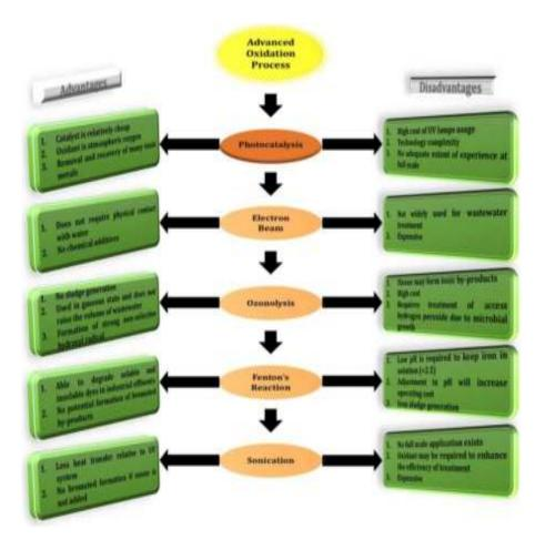
Figure 2 Merits and demerits of advanced oxidation process
