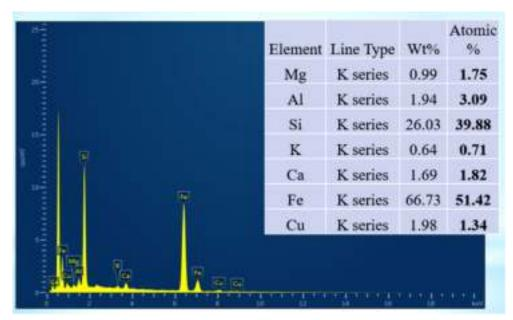
Figure 3 EDAX pattern and the corresponding elemental analysis of Cu-slag.
