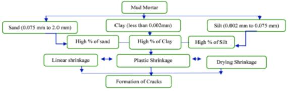
Figure 4 Consequences of improper composition of mud mortar [36,37]
