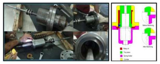
Figure 4 Lapping (step) marks observed on the mating surfaces of trip piston and spring holder
