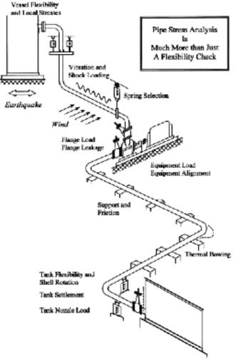
Figure 1 Tasks of pipe stress analysis
