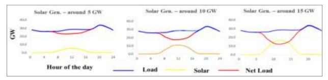
Figure 4 Change in net load due to different levels of VRE (solar) deployment
