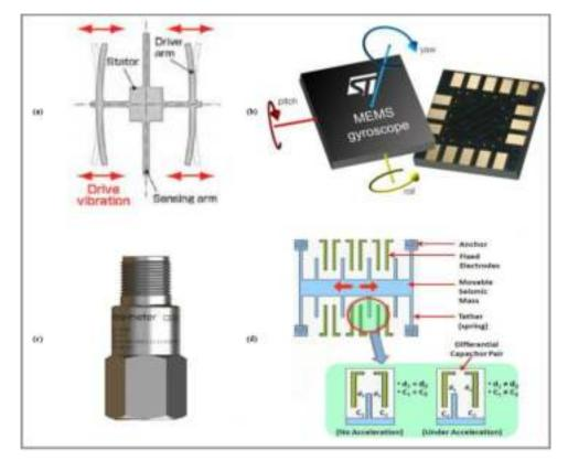
**Figure 3** Gyro and accelerometers sensors on the market : (a) Vibration Gyroscope; (b) MEMS Gyroscope; (c) Piezoelectric Accelerometer; (d) MEMS accelerometer
