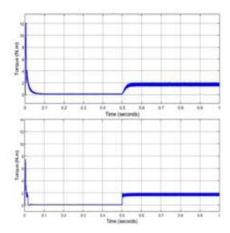
Figure 4 Torque waveform (a) open loop (upper) (b) closed loop with converter (lower)
