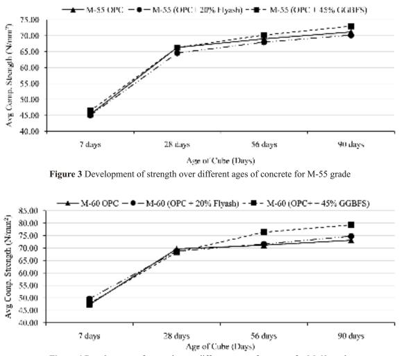
Figure 4 Development of strength over different ages of concrete for M-60 grade
