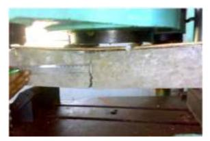
Figure 10 Flexural strength test
