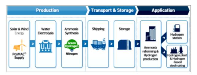
Figure 3 Supply chain for green hydrogen
