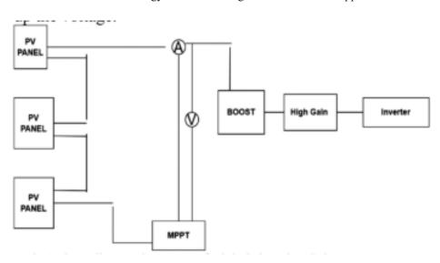
Figure 1 Overall control strategy of high gain DC-DC converter
