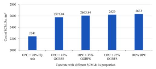
Figure 9 Comparison of cost of concrete of M-50 grade with different SCM
