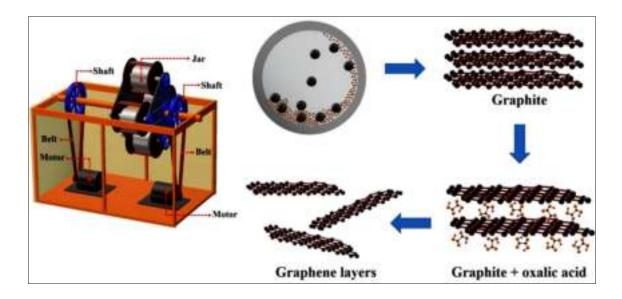
horizontal planetary ball mill having stainless steel jar and hardened steel balls. Oxalic acid and toluene are used as process control agents and milling medium. This is a comparative study as well, where the graphene obtained by milling both natural flaky graphite from ore as well as commercially available graphite powder are compared, to study the extent of exfoliation in both type of samples.
