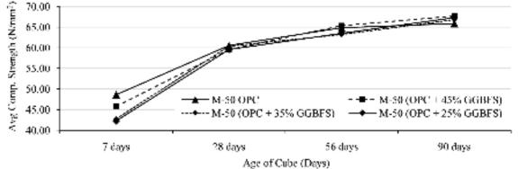
Figure 5 Development of strength over different ages of concrete for M-50 grade with different proportion of GGBFS and compared with OPC concrete
