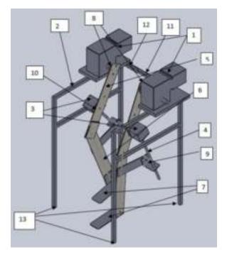
**Figure 12** Final 3D CAD model assembly of the device 1. Stepper Motor, 2. Stand, 3. Stepper Motor, 4. Lead Screw, 5. Upper Link, 6. Lower Link, 7. Ankle and Foot Support, 8. Flange Coupling, 9. Lower link Bracket, 10. Upper link Bracket, 11. Adjustable link Middle, 12. Adjustable link Right (Left), 13. Position for Wheels (4 nos)
