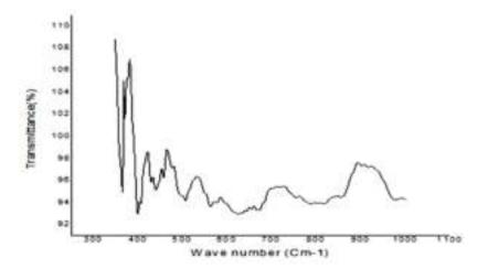
Figure 8 FT-IR analysis of the mud mortar sample
