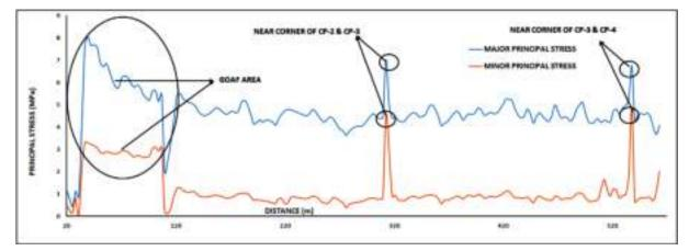
Figure 15 Principal stress distribution on the main gate (MG-1)
