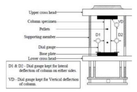
Figure 5 Schematic diagram of test setup
