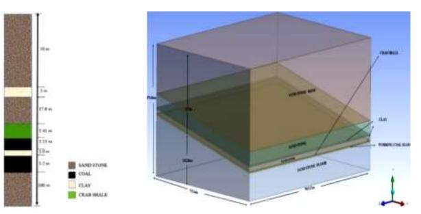
**Figure 2** Lithology of the mine site used for finite element model
