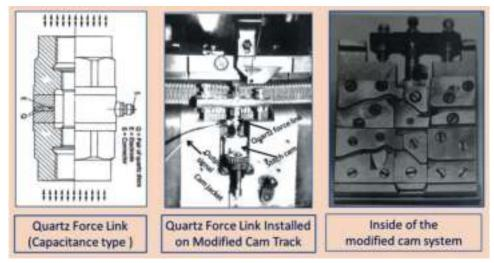
Figure 1 Sensor fitted on the stitch cam of the new cam track
