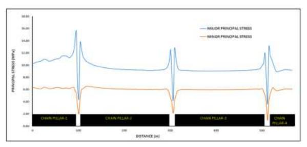
Figure 14 Principal stress distribution on the chain pillars
