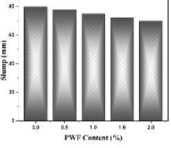
Figure 4 Slump vs PWF content
