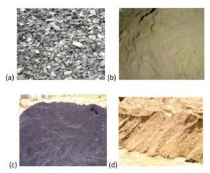
Figure 1 (a) Coarse aggregates (b) Cement (c) Copper slag and (d) River-sand used for experiments
