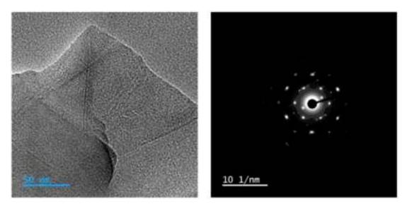
Figure 6 TEM image and SAED pattern of ore graphite
