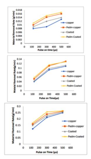
Figure 2 Effect of pulse -on -time on MRR at (a) 6 A (b) 9 A (c) 12 A current
