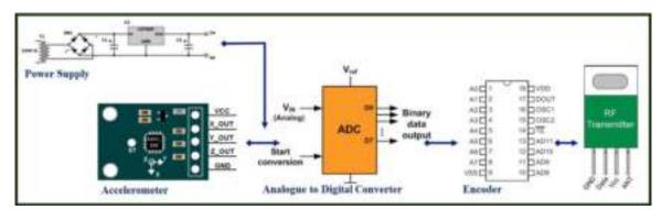
Figure 5 Transmitter circuit for gesture controlled vessel
