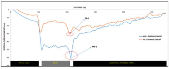
Figure 10 Vertical displacement distribution in gateroads
