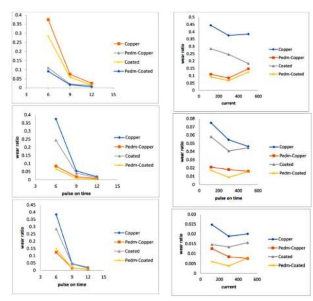
**Figure 3** Effect of current on wear ratio at (a) 120µs (b) 300 µs (c) 500 µs pulse -on-time
