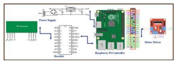
Figure 6 Receiver circuit for gesture controlled vessel
