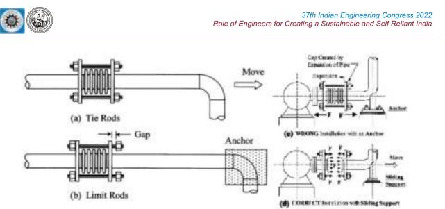
Figure 6 Bellow-type expansion joint installation considerations [1]
