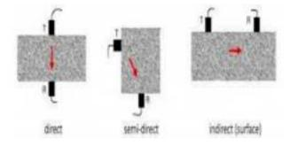
Figure 5 Methods of ultrasonic pulse velocity test
