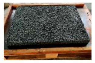
Figure 2 Pervious concrete
