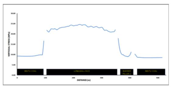
Figure 11 Vertical stress distribution on longwall working face
