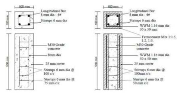
Figure 2 Reinforcement Detail of Control and Retrofitted Specimen
