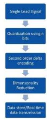
Figure 1 Signal flow diagram of lossless compression
