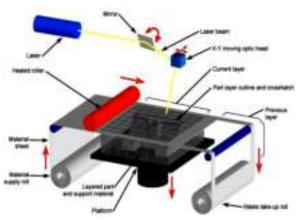
Figure 6 Laminated object manufacturing
