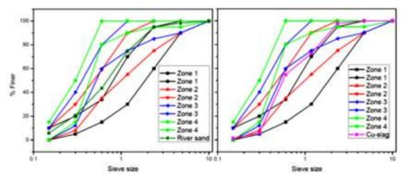
Figure 2 Semi log graph showing the sieve analysis of river sand (a) and Cu-slag (b)
