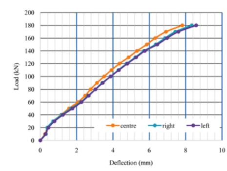
Figure 1Graphical representation of load vs Deflection for M7-SCC Mix
