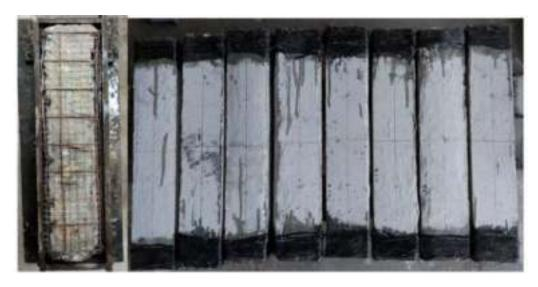
Figure 3 Reinforcing cage and wrapping of weld wire mesh
