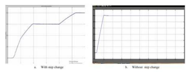
Figure 13 Motor Speed Waveform for conventional PI Controller
