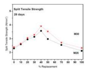
**Figure 6** Split tensile strength with percentage replacement of Cu-slag in river sand for mix designs M25 and M30 after 28 days of curing
