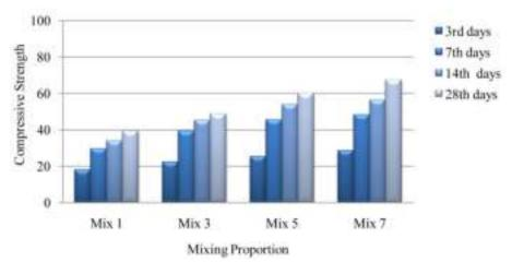
Figure13 Comparison between the compressive strength for the ratio of M60
