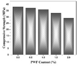
Figure 5 28-day Compressive strength vs PWF content
