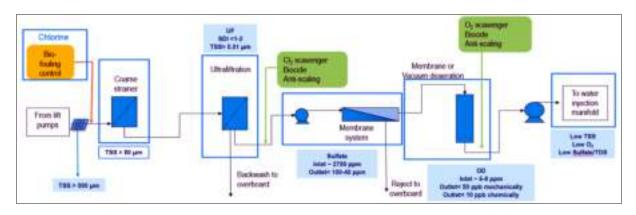
Figure 2 Overview of waterflood injection
