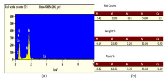
Figure 6 (a)SEM with EDAX image (b) Quantification of the constituents of the mud mortar sample
