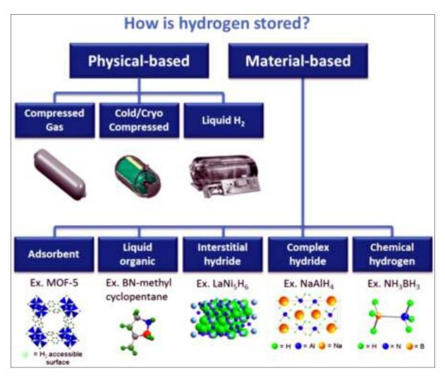
Figure 4 Various methods of storage of hydrogen
