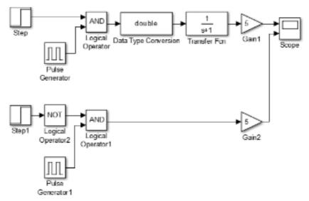
Figure 4 Timer design through Simulink
