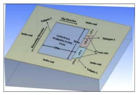
Figure 4 Longwall panel showing the chain pillars, gateroads and face gallery at setup room
