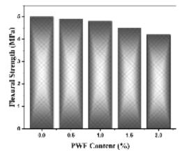
Figure 6 28-day Flexural strength vs PWF content
