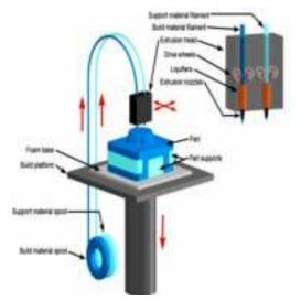
Figure 5 Fused deposition modeling
