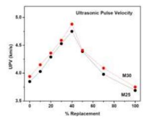
Figure 8 Variation in ultrasonic pulse velocity of concrete cubes casted with varying percentage replacements of Cuslag in river sand for mix designs M25 and M30 after 28 days of curing
