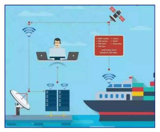
Figure 4 IoT application: automatic identification systems for a marine vessel[23]
