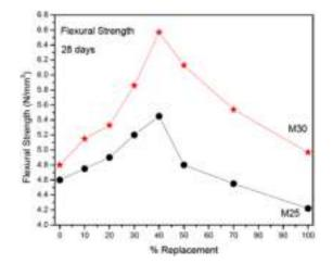
**Figure 7** Variation in flexural strength with percentage replacement of Cu-slag in river sand for mix designs M25 and M30 after 28 days of curing
