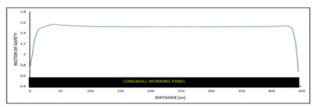
Figure 17 Safety factor distribution of the longwall panel
