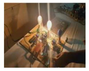
Figure 4 Demonstration of automatic cutoff of one load during power cut
