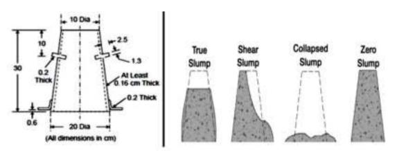
Figure 8 Slump test of geopolymer concrete
