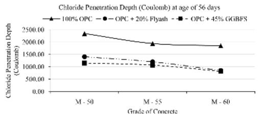
Figure 7 Chloride penetration of different grades of different concrete at 56 days
