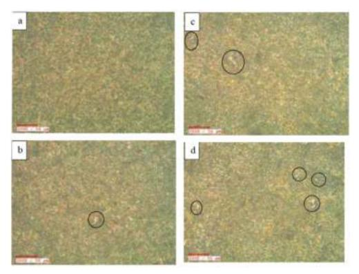
**Figure 2** Microstructure images of (a) Unreinforced AA6061, (b) 2.5%, (c) 5% and (d) 10% steel reinforced AA6061 at 200X magnification
