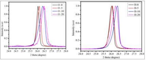
Figure 2 Normalised XRD of ore and commercial graphite
