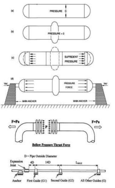
Figure 5 Bellows pressure thrust and restraining arrangement [1] [6]
