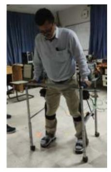
Figure 13 Final prototype of hip-knee exoskeleton
