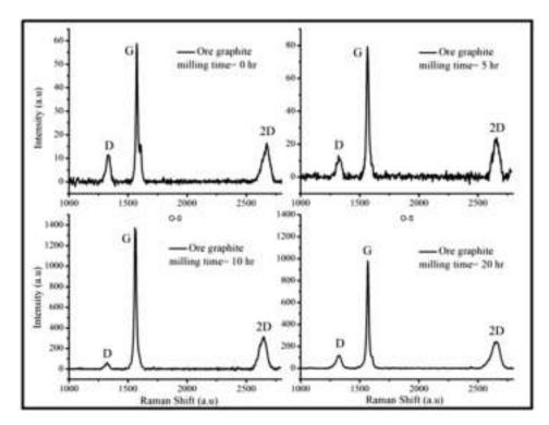
Figure 3 Raman spectrum of ore graphite
