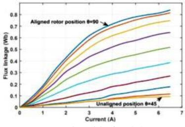
Figure 2 Characteristics of SRM [13]
