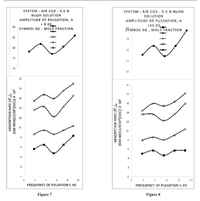
Increase in splashing may be reducing mass transfer rates it was experimentally observed that liquid splashing increased with the increase of amplitudes[1].
