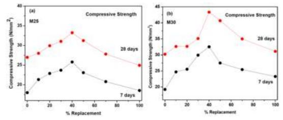
**Figure 5** Compressive strength with varying percentage replacements of Cu-slag in river-sand for mix designs M25 and M30 after (a)7 days and (b) 28 days of curing
