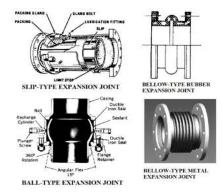
Figure 1 Different constructions of expansion joints
