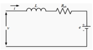
Figure 1 Single phase equivalent circuit of SRM [8]
