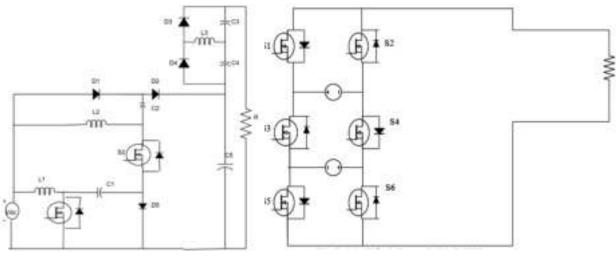
Figure 2 Interleaved non -isolated quadratic DC-DC converter[9]
