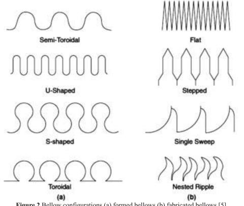
Figure 2 Bellow configurations (a) formed bellows (b) fabricated bellows [5]
