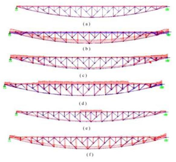
**Figure 5** (a) Stress diagram for Stage 1; (b) Stress diagram for Stage 2; (c) Stress diagram for Stage 3; (d) Stress diagram for Stage 4; (e) Stress diagram for Stage 5; and (f) Stress diagram for Stage 6
