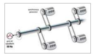
Figure 2 The concept of synchronous generators working together in an electrical grid
