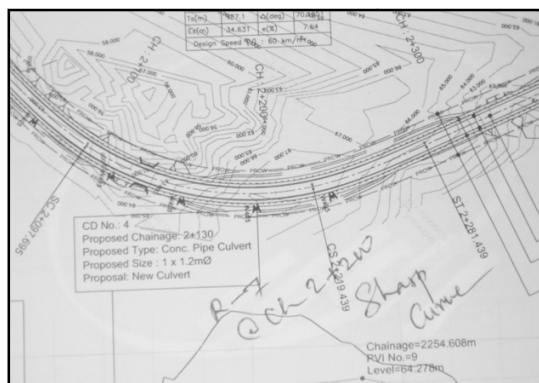
Figure 1 Example of a sharp curve in design drawing
