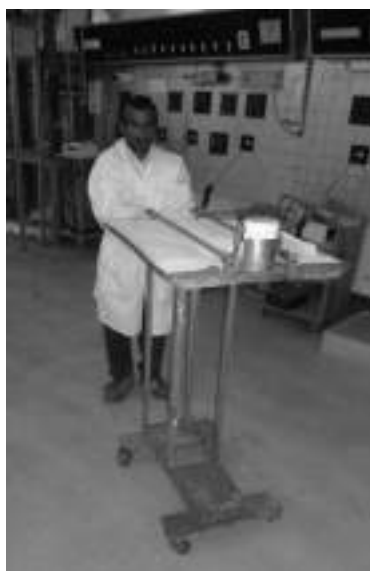
Figure 1 Device for unlocking the hook toggle clamp of the lead pot LP-30 used for transportation of I-131 sodium iodide solution
