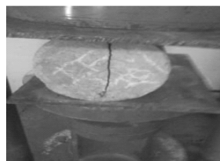
Figure 10 Cylinder specimen after failure
