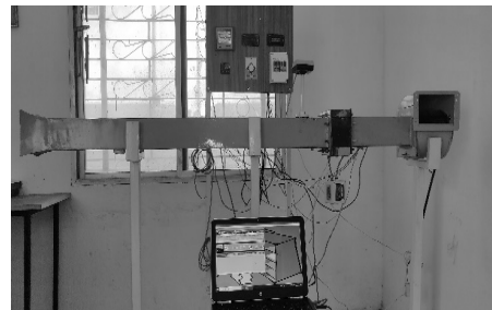
Figure 2 Experimental Setup with sensors and Data Logger (ASME Standards MFC-26-2011)
