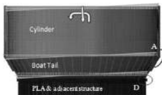
Figure 3 FE model of PLF with loads and BC
