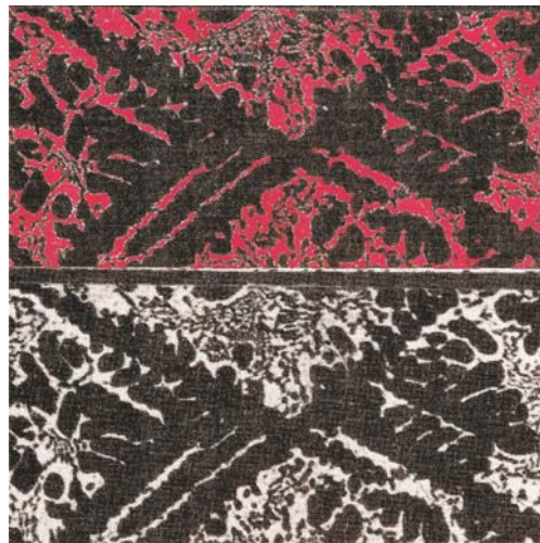
Pic. A Cooper dendrites in copper silver eutectic x 80
