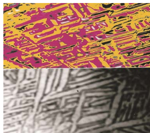
Pic. E Martensite needles in austenite x 1200
