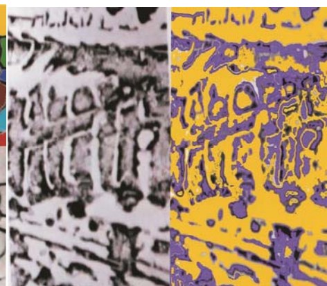
Pic. D Hypoeutectic case iron x200
