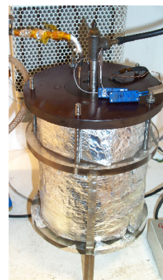
Fig. 1 Schematic diagram of reaction vessel within the calorimeter. picture of the calorimeter installed with air and nitrogen flow inlet and outlet, thermocouples connected to data acquisition and temperature control unit
