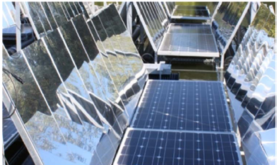
Fig. 2 The floating tracker cooling concentrator (FTCC) design, Italy [1]
